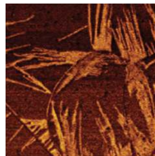
CdTe nanowires. Topography image (top), surface potential (bottom). Scan size 2 \mu\text{m} .
